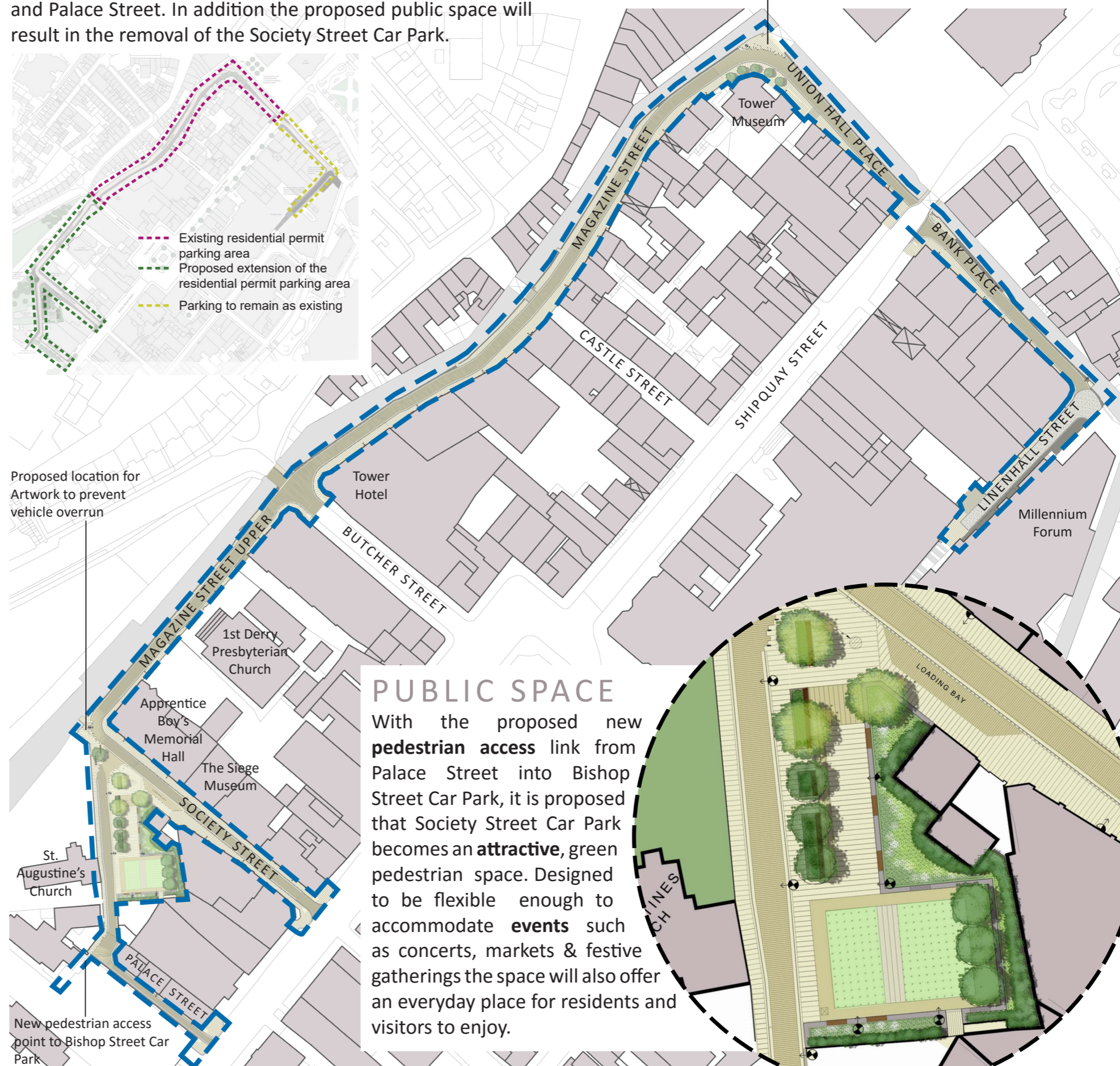
Proposed location for Artwork to prevent vehicle overrun. Demountable bollards/artwork will be included for service/emergency access through Magazine Gate.
